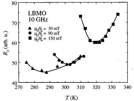
FIG. 1. Temperature dependence of the surface resistance at 10 GHz of a LBMO ceramic for fields of 30 mT (triangles), 90 mT (circles), and 150 mT (squares). The minima correspond to point where Eq. (3) is satisfied.
