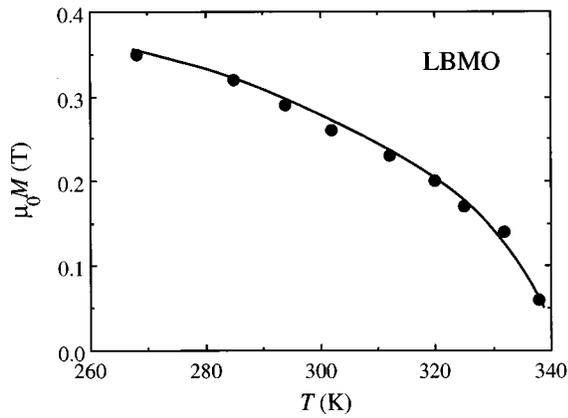
FIG. 2. Temperature dependence of the magnetization of a ceramic LBMO sample. The magnetization was inferred from Eq. (2).
