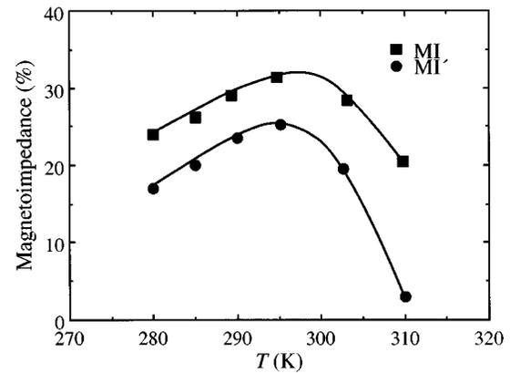
FIG. 3. Temperature dependence of the magneto-impedances MI and MI' at 30 mT for a sintered LBMO sample at 10 GHz. MI, which reaches its maximum near 300 K, is the more meaningful quantity since the sample is measured in a monodomain state.
