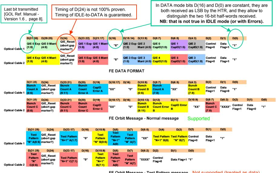
FE Orbit Message - Test Pattern message Not supported (treated as data)
