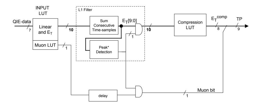
In case that after the summing there is a "plateau" [e.g.: 0, 10, 10, 0] select all the relative maximum points. In HF the pulse is faster and there is no need to do the L1 filter.
