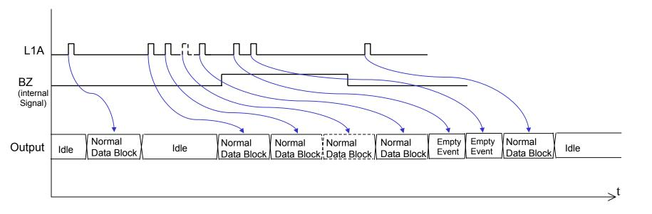
Note that the BZ included in each Data Block, latches the value of the internal BZ at the beginning of each block transmission.
