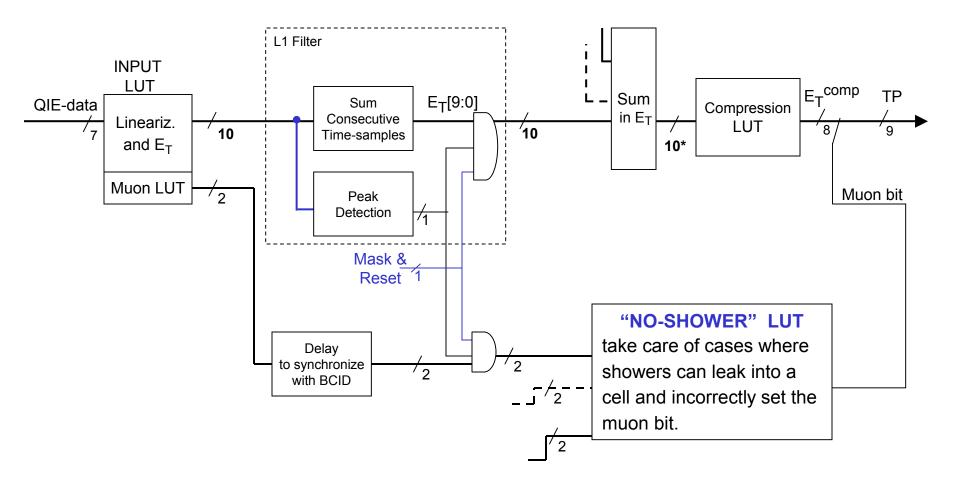
\* If overflow, set the result to the max value. Investigate 11-bit sum and LUT. Note that there is a unique compression LUT for a group of channels. Each channel participating on the sum must have the possibility to be masked, to perform a sync histogram based on each independent channel (input data from each deserialiser) [Carlos]
