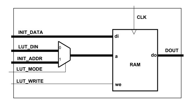
NB: during configuration this LUT has non-zero outputs, so need to disable (Stop command) the SLB board (software specification).
