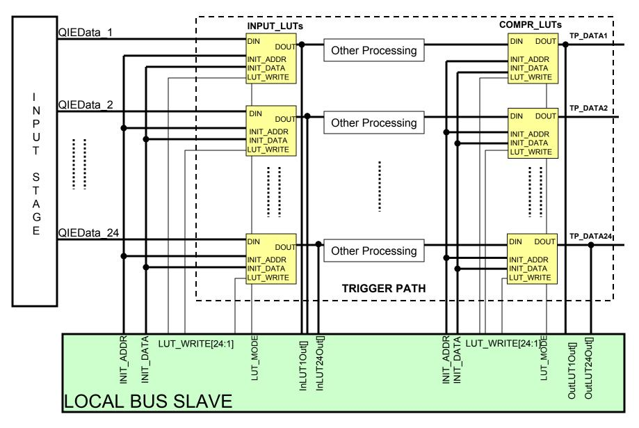
NB: to configure a given LUT, from VME the access will be always at the same address. Then on the board VME FPGA the correct address will be generated with a counter.
