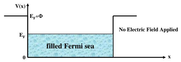
If an electric field is applied to the surface of a metal, the potential is modified and it becomes possible for electrons to tunnel out of the metal into free space (this is called cold emission by Fowler-Nordheim tunneling).
