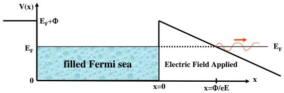
Note that the tunnel barrier is not a "flat top" but instead triangular shaped. The potential is given by  $V(x) = E_F + \Phi - eEx$ , where E now (confusingly!) is the applied electric field. The calculation of the Fowler-Nordheim tunneling rate is a job for the WKB approximation!
