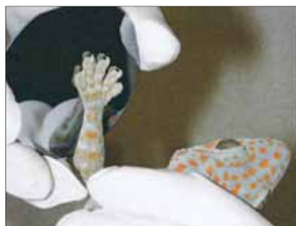
Figure 6. The strong adhesion between the hydrophobic surface of tokay gecko toes and the molecularly smooth, hydrophobic surface of a wafer of gallium arsenide demonstrates that the van der Waals force is a sufficient mechanism of gecko adhesion. (Photograph courtesy of the author.)
