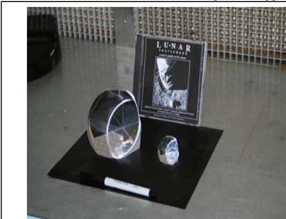
Figure 4 The 100 mm CCR fabricated to demonstrate the capability to meet the required specifications next to one of the CCRs from the Apollo project.
