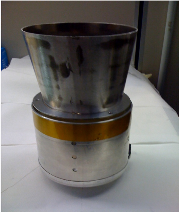
Fig. 11. This is a hardware implementation of the current LLRRA-21 package design. This unit, with the sun shade, was tested in the thermal/optical/vacuum system in Frascati in April 2010.
