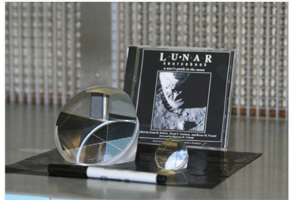
Fig. 1. Shows the Flight Certified 100 mm CCR that has been fabricated to the specifications with Apollo CCR. The offset angles for the back faces significantly exceeded the specifications, for two of the angle by almost a factor of two.
