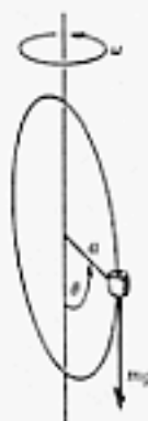
Fig. 9.9 A bead sliding on a rotating hoop.
