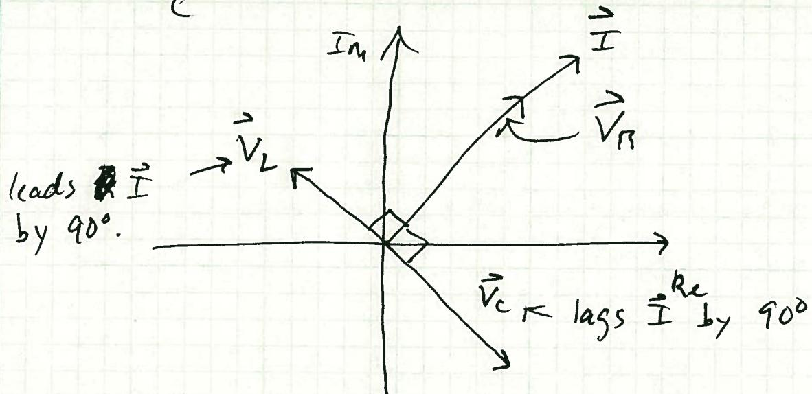
Voltage Loop Rule:  $\vec{V}_S = \vec{V}_R + \vec{V}_L + \vec{V}_C$
