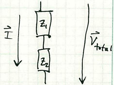
$$\therefore \vec{V}_{\text{total}} = \vec{I}(Z_{\text{series}}) \quad \text{where } Z_{\text{series}} = Z_1 + Z_2.$$
