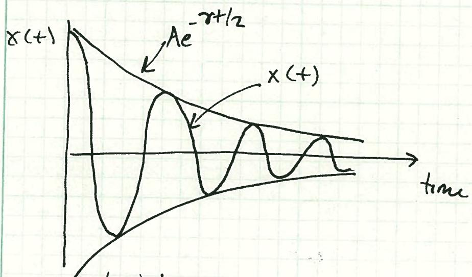
The mechanical energy of the oscillator is being converted into heat by the drag force.
