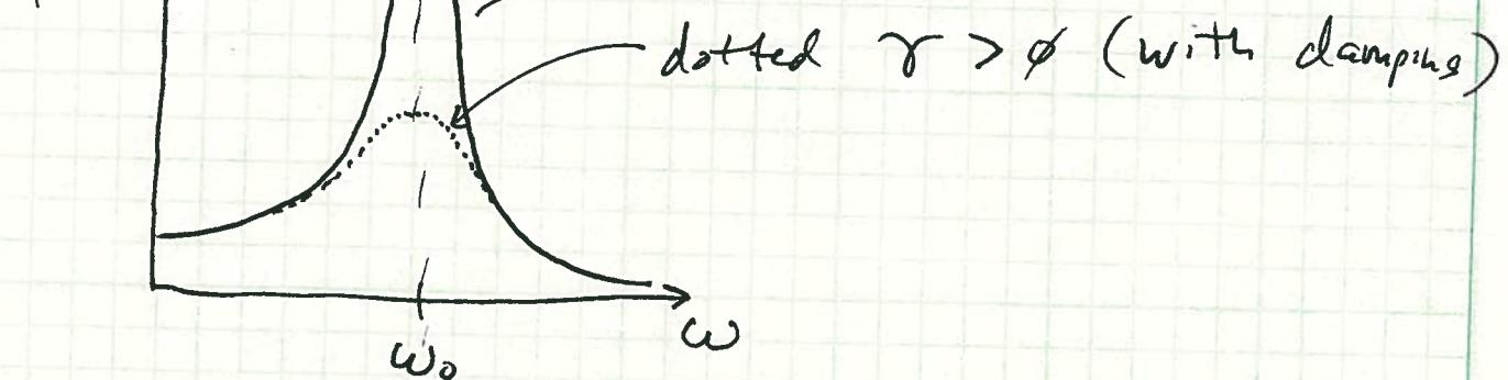
An ideal oscillator with no damping has an infinite amplitude at  $\omega = \omega_0$ . But this never happens in nature, because there is always some damping.
