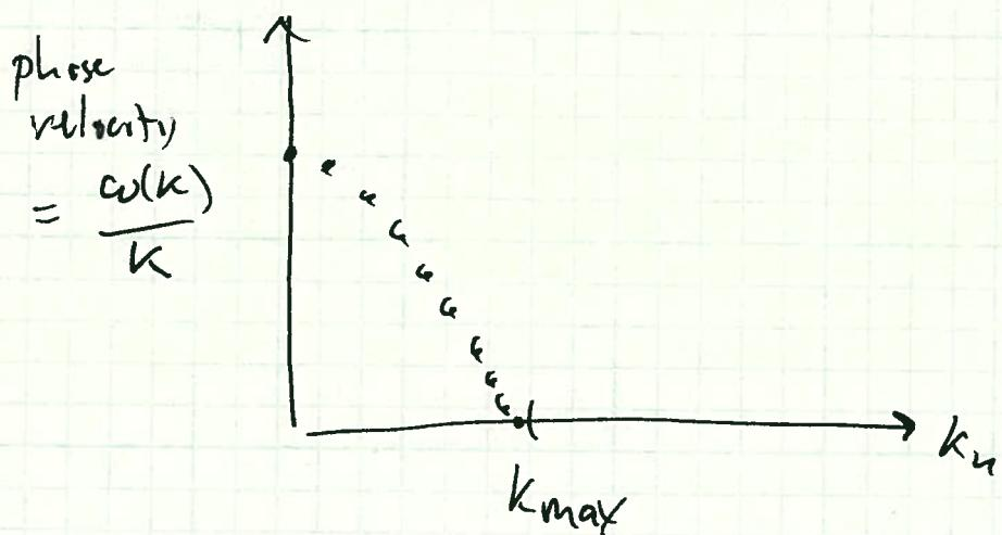
The  $\omega(k)$  function is called the "dispersion relation", and the ratio of the dispersion relation and  $k$  is the phase velocity. The dispersion relation for the classical wave equation is
