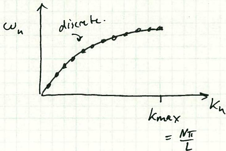
The reason why this system does not have a linear relationship between  $\omega$  &  $k$  is because its equation of motion is not the simple classical wave equation. Its equation is
