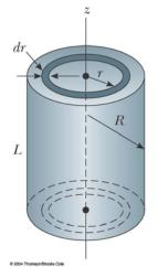
Keep in mind this a cylindrical shell with a middle section and two ends at the top and bottom. You need to include the contributions from the top and bottom pieces in your answer. Also, assume that the amount of mass distributed on the body of the cylinder, the top of the cylinder and the bottom of the cylinder are each M. So, the body has mass M, the top has mass M and the bottom has mass M.
