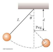
a) If the pendulum is released from  $\theta = 90^{\circ}$ , the length of the string L is equal to 5/3m and in the course of its motion, the mass swings in a complete circle around the peg. What is the minimum value for d?
