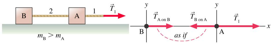
$$m_{A}: \sum F_{A} = T_{1} - T_{BA} = m_{A}a, \ m_{B}: \sum F_{B} = T_{AB} = m_{B}a,$$
