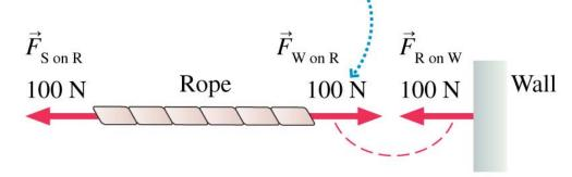
Imagine cutting the rope in two pieces. There are two forces on the left half of the rope:
