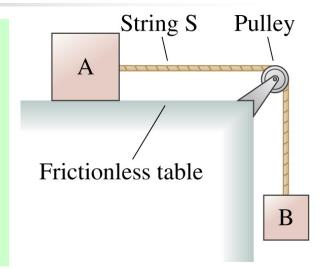
A *massless* rope around a *massless* pulley cannot have a net force acting on it. So if it is *frictionless*, the tension forces pulling its two ends must cancel each other *as if* they form an action-reaction pair.
