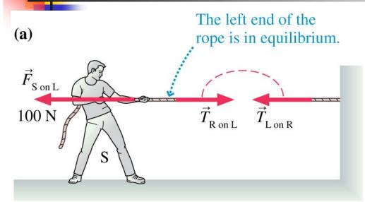
The wall pulls on the rope with a force of 100 N.
