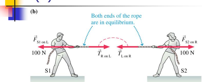
The left half of the rope has the same forces on it as in the wall case:  $T_{RL} = 100 \text{ N}$ . There are two forces on the right half of the rope, and the rope doesn't accelerate:  $100 \text{ N} - T_{LR} = 0$ ,  $T_{LR} = 100 \text{ N}$ .
