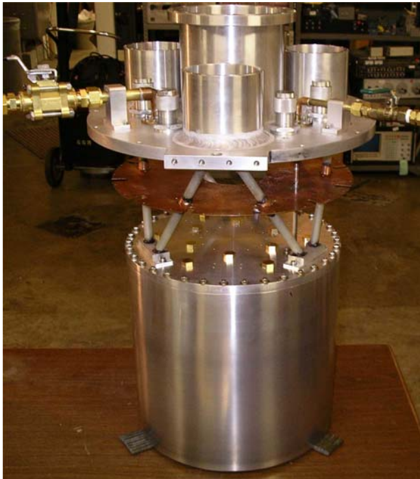
Fig. 6. The partially assembled cryostat showing the fiberglass strut structure supporting the SGG vacuum can.
