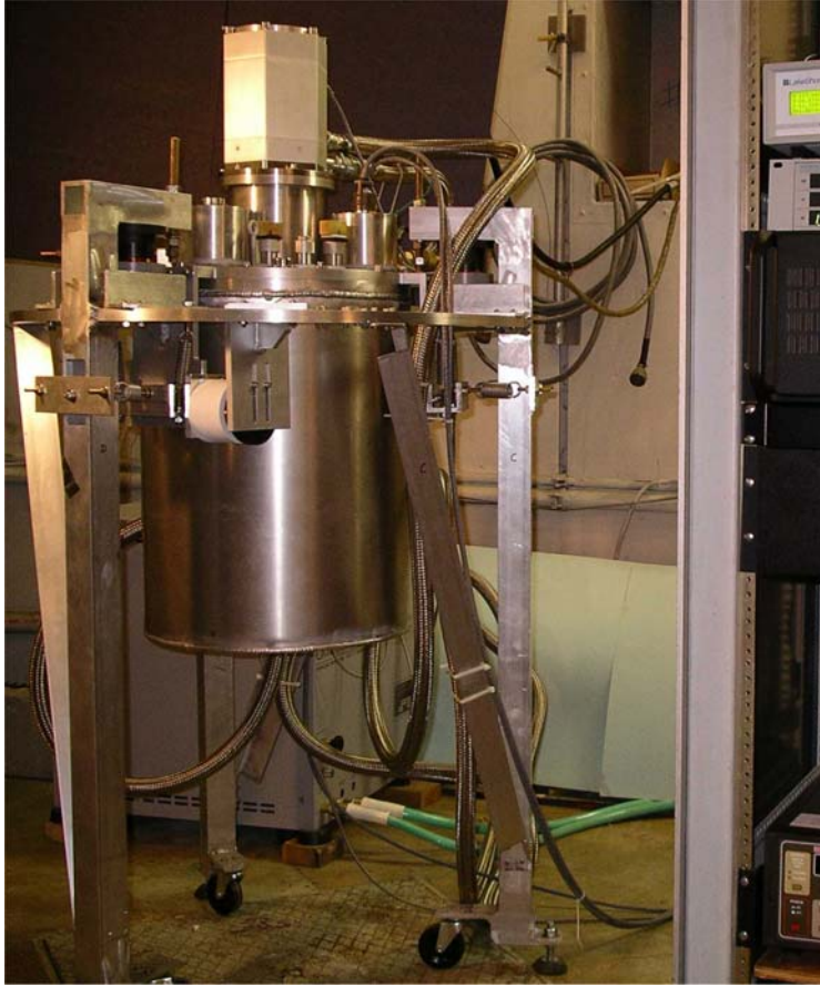
Fig. 7. The assembled cryostat on the support structure.
