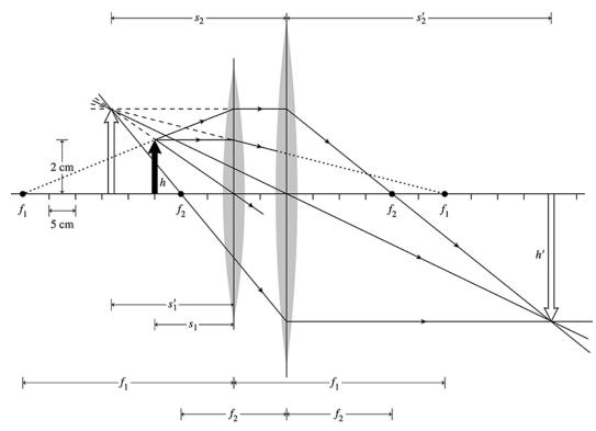
The figure shows the two lenses and a ray-tracing diagram. The ray-tracing shows that the lens combination will produce a real, inverted image behind the second lens.
