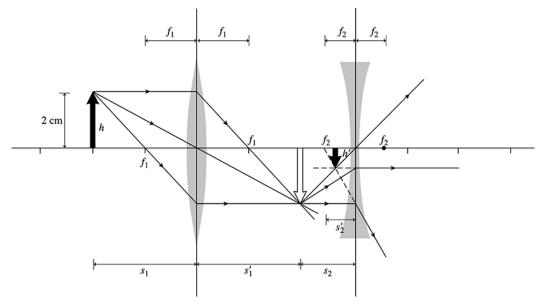
The figure shows the two lenses and a ray-tracing diagram. The ray tracing shows that the lens combination will produce a virtual, inverted image in front of the second lens.
