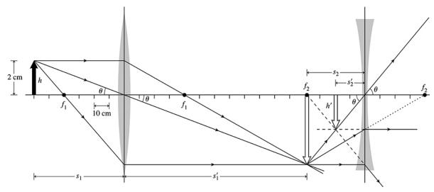
The figure shows the two lenses and a ray-tracing diagram. The ray tracing shows that the lens combination will produce a virtual, inverted image in front of the second lens.
