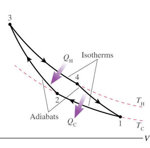
• work during 4 processes; heat transferred during 2 isothermal...
