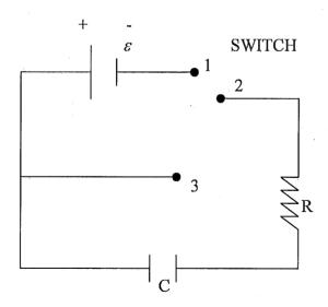
At t=0, connect 1 to 2: charge will flow from battery to capacitor plates.
