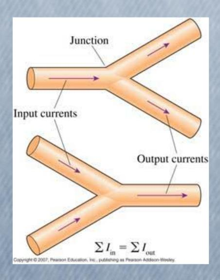
The sum of currents into a junction must equal the currents flowing out of it
